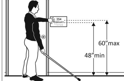
Note: If the sign is at double doors with one active leaf, the sign should be on the inactive leaf; if both leaves are active, the sign should be on the wall to the right of the right leaf.
